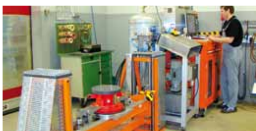
Figure X3: PROTEGO® Vent Valve „Bubble“ Testing
